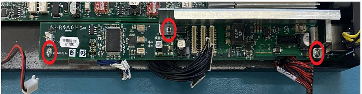
**Picture 6.11** Baffle Plate and Control Card Screw Locations
