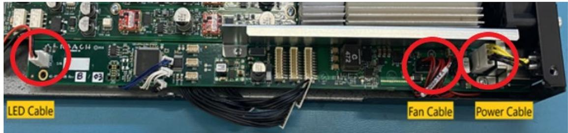
**Picture 6.12 Fan, LED, and PWR Connection Locations**
