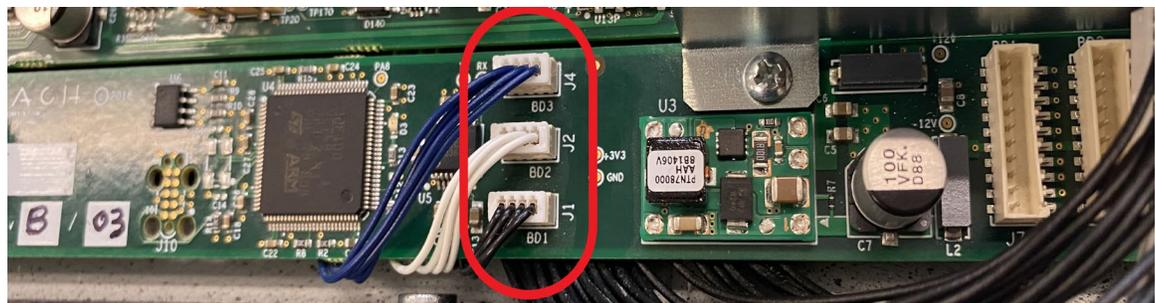
**Picture 6.13 Line Card 4-pin Cable Locations**
