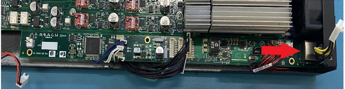
**Picture 6.9** Installing the New Control Card
