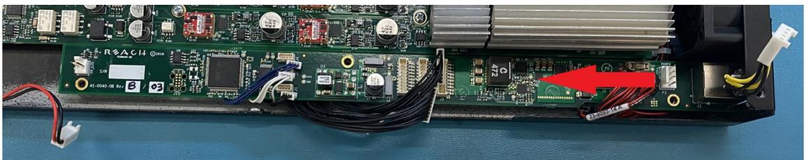
**Picture 6.8 Control Card Removal Direction**
