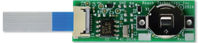
RTC Module with Battery and Cable Installed.
