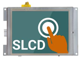
deeper blacks and, by extension, better picture quality and a wider viewing angle (80/80 left/right, 80/80 up/down vs. 80/50 left/right, 60/60 up/down). Please let us know if you require a first article to confirm your acceptance of the new part. See the <u>new panel</u> specification.
