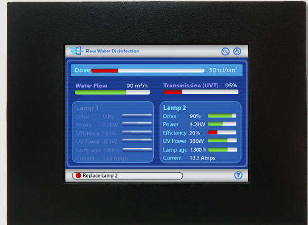
5.7-inch High Resolution Enclosed Unit, front view
