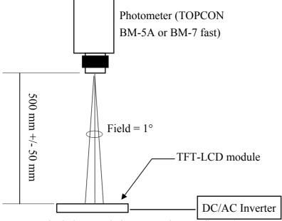
Optical characteristics measuring configuration Note 12-5: The uniformity of LCD is defined as
