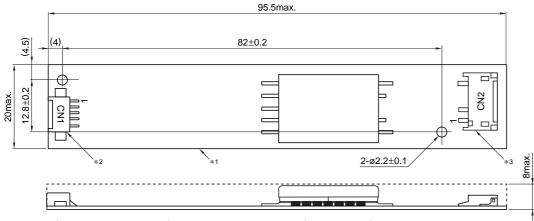
\*1Substrate(PWB: Printed wiring board): Inflammable material UL94V-0(FR-4 or CEM-3) t=1mm
